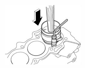
Apply liquid gasket to the oil seal case and install the oil seal case(A).
