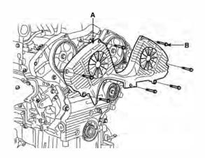
10. Remove the drive belt idler pulley(A).
