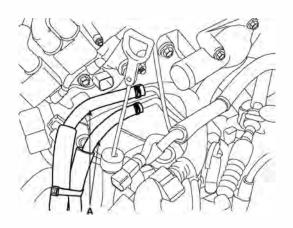
21. Disconnect the ABS wheel speed sensor(A) from both front knuckles. (See DS group - front axle).
