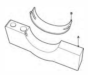
5. Install thrust bearings.
