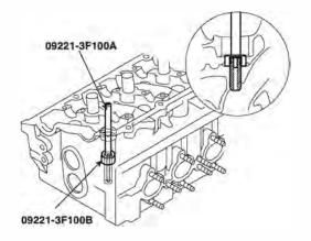
3. Using the SST(09221-3F100A/B), press-fit the valve guide. The valve guide must be press-fitted from the
