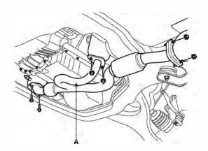
5. Remove the exhaust manifold(A) and gasket(B).
