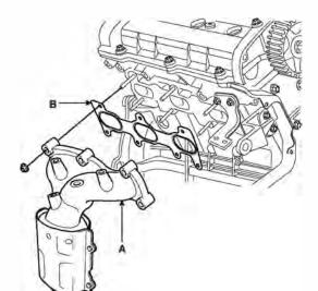
4. Install the front exhaust pipe(A).
