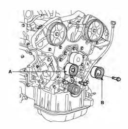
4. Align the timing marks of the camshaft sprocket and crankshaft sprocket with the No.1 piston placed at top dead center and its compression stroke.
