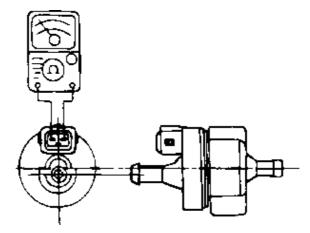
Measure the resistance between the terminals of the solenoid valve.
