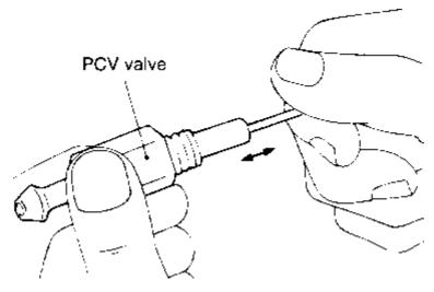
If the plunger does not move, the positive crankcase ventilation valve is clogged. Clean it or replace.
