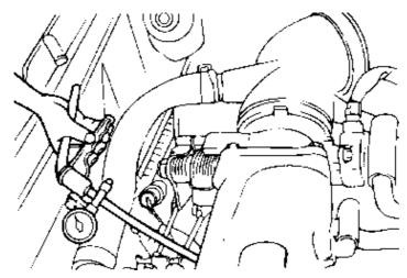
Start the engine and check that, after raising the engine speed by racing the engine, vacuum remains fairly constant.
