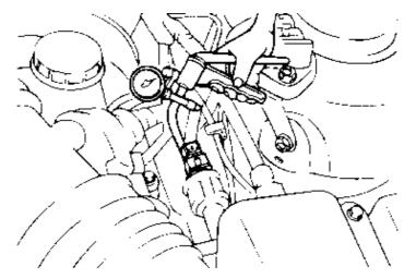
Apply vacuum and check when voltage is applied to the evaporative emission canister purge solenoid valve and when the voltage is discontinued.
