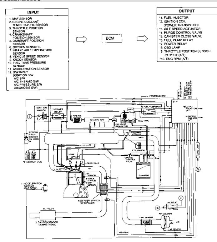
ECM : Engine Control Module OBD : On Board Diagnosis MAF : Mass Air Flow Sensor A/C : Air Conditioning
