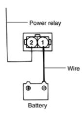
Inspect that CCV is close when attaching the wire to (-) of battery.
