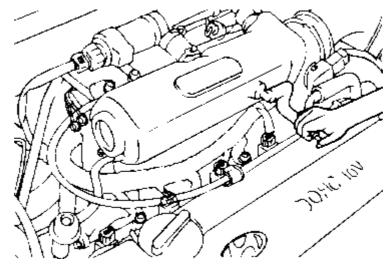
Run the engine at idle and put a finger on the open end of the PCV valve and make sure that intake manifold vacuum is felt.
