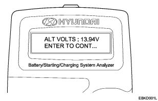
3. Turn off all electrical load and rev engine for 5 seconds.
