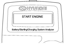
Cranking voltage and starter test results will be dis-
