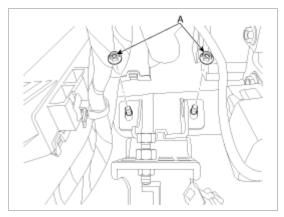
7. Remove the clutch master cylinder from the clutch pedal assembly by rotating the clutch master cylinder 45 degree counter clockwise.
