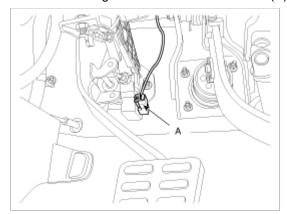
4. Remove the push rod from the clutch pedal by removing the snap pin (A) and washer (B).
