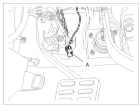
6. Install the flexible hose (A) to the brake reserve tank.
