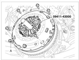
3. Loosen the bolts(6ea) which attach the clutch cover to the flywheel in a star pattern. Loosen the bolts in succession, one or two turns at a time, to avoid bending the cover.
