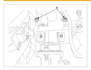
3. Install the clutch pedal mounting nut (C-3ea).
