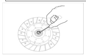
2. Install the clutch disc assembly to the flywheel using the special tool (09411-43000).
