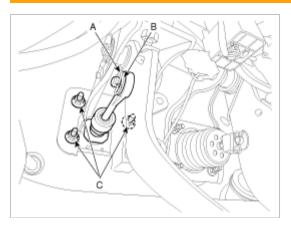
4. Install the push rod to the clutch pedal by installing the snap pin (A) and washer (B).
