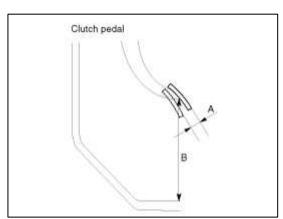
2. If the clutch pedal freeplay and height is not within the standard value range, adjust as follows:
