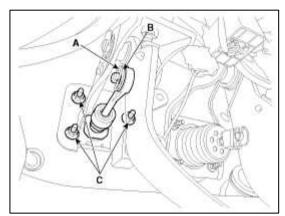
4. Install the push rod to the clutch pedal by installing the snap pin (A) and washer (B).
