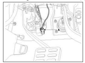
6. Install the flexible hose (A) to the brake reserve tank.
