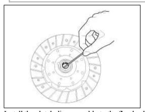
2. Install the clutch disc assembly to the flywheel using the special tool (09411-1P000).
